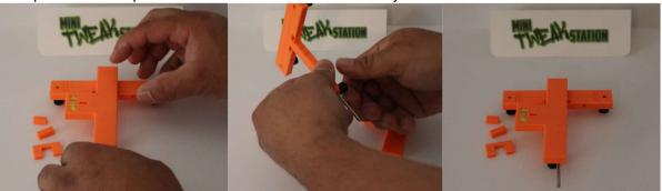
Verify that it's level one more time from side to side and front to back. IMPORTANT: Make note of the contact points of the thumb turns on your working surface. Any relocation from these contact points will require the "T" to be leveled again to this new area.
