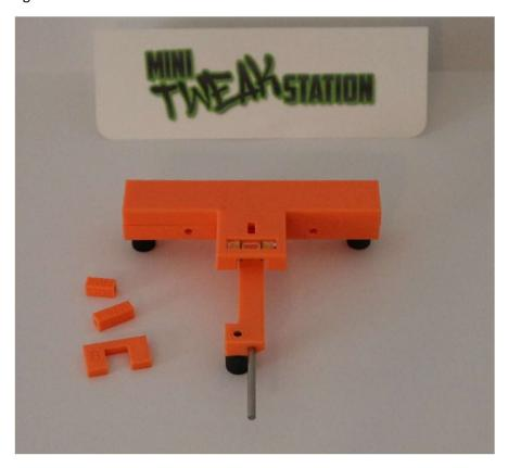
Determine if your wheelbase is 98mm or 102mm and slide the appropriate wheelbase spacer onto the guide rod.
