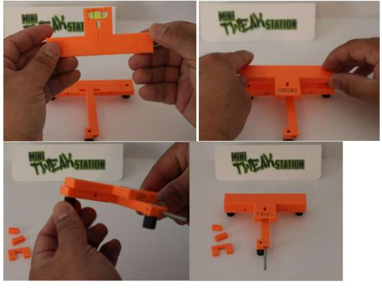
Now place the level parallel with the shaft of the "T" and adjust the thumb turn on the shaft until it is level front to back.
