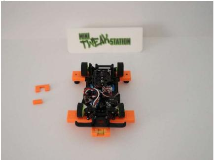
Gently tap the center of the rear suspension, either on the screw of the disk damper, the chassis connection of your tridamper or the top shock. Tapping the rear suspension causes it to naturally settle.
